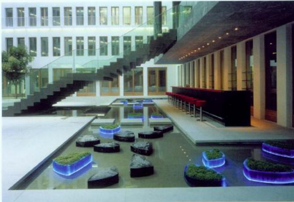
The glass lenses were fused in split molds out of white and blue ARTISTA®
