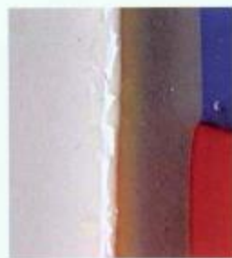
Flaked edge resulting from change in crystal structure.
