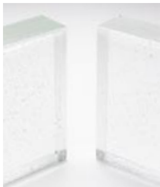
1401-30F, right, for crystal clarity. Tekta Clear, left, for cost savings. Slabs are 1 3/4" thick, fused from 14 layers of 3mm sheet glass.
